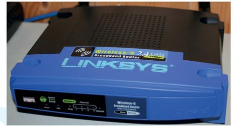
OpenWrt started life on Linksys' original WRT54G (the later WRT54GL show here), and used the GPL code released by Linksys [image: CC BY-SA Vidarlo ENWP]
