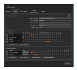
Our audio device has 20 individual inputs and outputs, but Bitwig is able to make sense of this configuration with only a little help from us.
