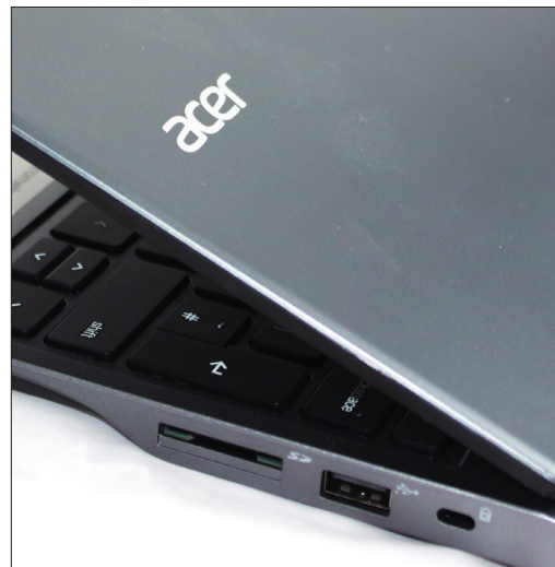
There's a USB 2 port and a USB 3 port, plus an SDCARD reader – but there's only 10GB of usable local storage.
