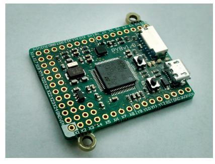
The Pyboard measures just 33 x 40 mm and weighs 6g. There's a tutorial at http://tinyurl.com/o529no5 that illustrates how easy it can be to use it with a servo.
