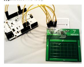
Hover also has five touch points: one in the centre of the board and the other four at the north, east, south and west edges of the board. This gives us nine methods of control for this small board.
