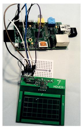
Hover easily connects to the Raspberry Pi using only six connections to the GPIO, enabling it to be integrated into your projects with minimal fuss.
